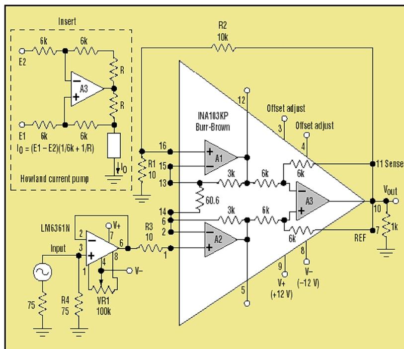
To attain 600-MHz gain-bandwidth, the output stage of the instrumentation amplifier is configured as a modified Howland-current pump.
