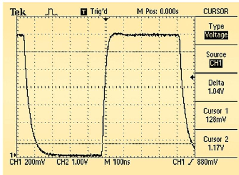
C. The peak in the waveform disappears when the conventional amplifier is properly terminated. But, note the change in vertical scale factor due to halving the amplitude.
