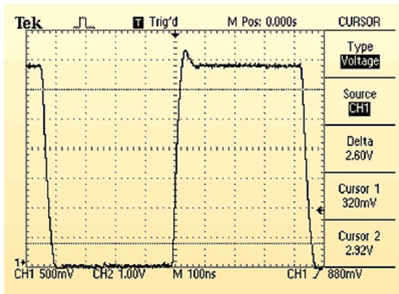
B. When unterminated, the waveform of the conventional amplifier measured at the far end of the coaxial cable exhibits a slight peak.
