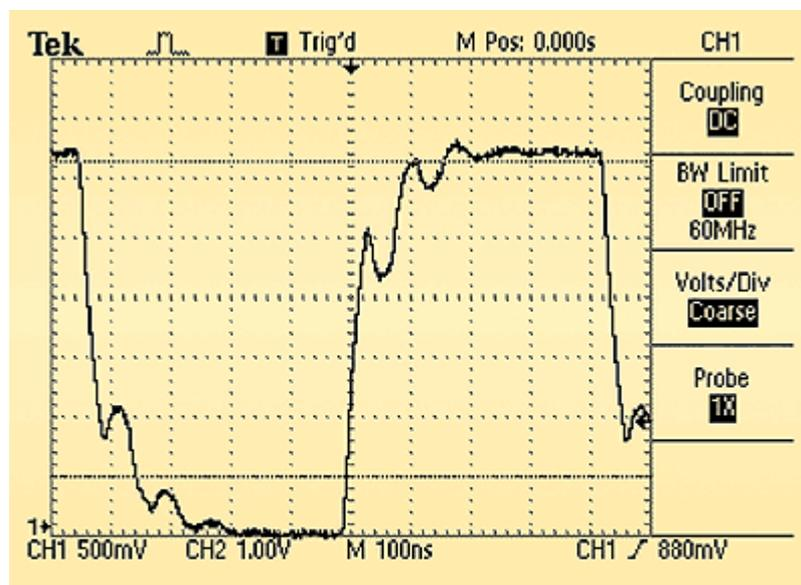
D. This waveform results when the active termination circuit isn't terminated. The poor signal fidelity is probably the result of using positive feedback under conditions it's not suited for.
