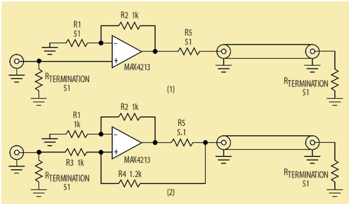
A. Two circuits were used to obtain the scope waveforms, a conventional circuit (1) and an active back-termination configuration (2). Notice that all of the waveforms are taken at the load (far) end of the 15 ft. of coax cable. RG-58 cable was used for these tests.
