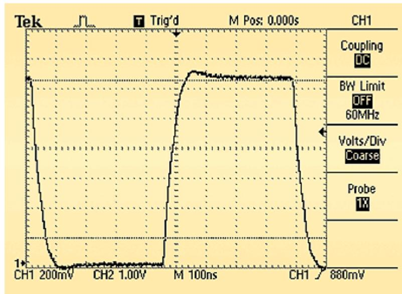
E. With the proper termination, the active termination circuit produces a much better waveform. Also, the waveform's amplitude isn't halved, as is the case when the conventional circuit is terminated.
