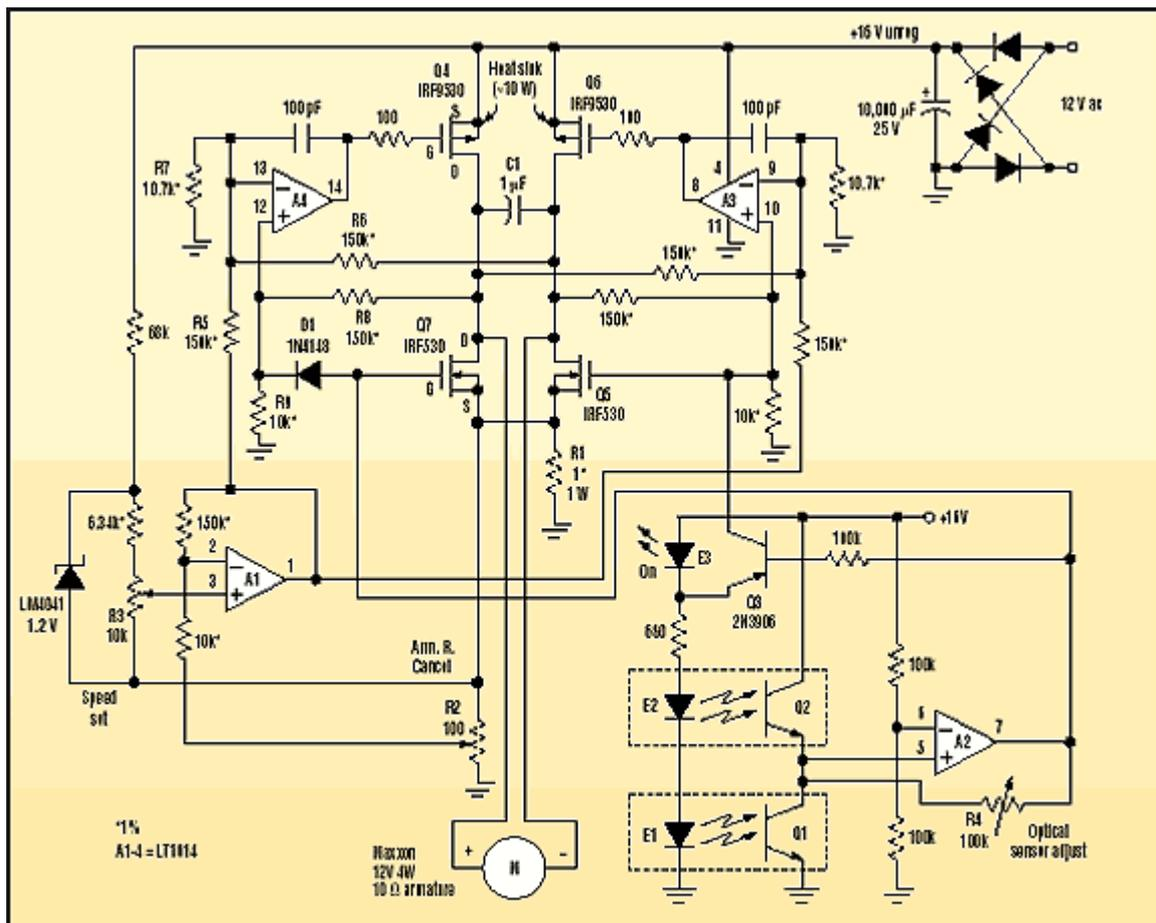
This circuit delivers motor-speed control by combining a motion-reversing H-bridge circuit topology with armature-resistance-cancellation circuitry.
