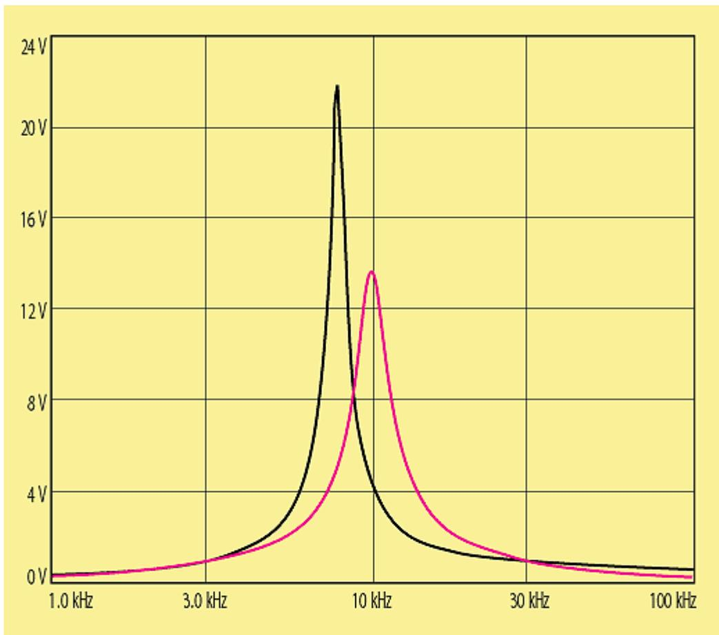
2. The bandpass filter response shows a 100% increase in Q. The 25% shift in the calculated center frequency can be compensated for in the design calculations.
