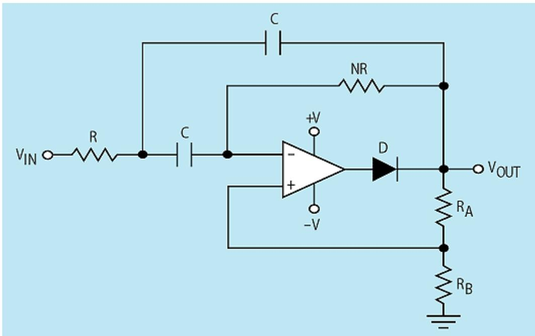
1. The single op-amp Delyannis bandpass-filter circuit is modified with the addition of a single diode at the amplifier's output. The diode increases the filter's Q by at least 100%.
